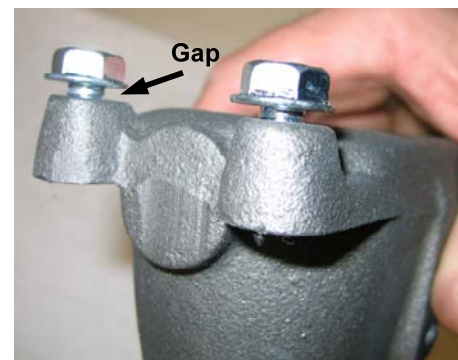
Figure 17: Leave a gap between the screw and the burner surface.
