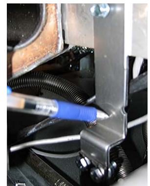
Figure 13: Install the gas manifold brackets. Ensure the notches are facing away from frypot.
