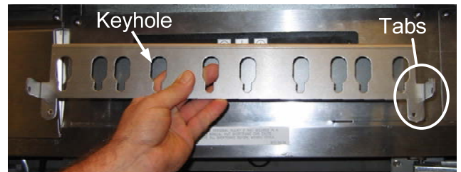
Figure 4: The brace in its final position, as it will look inside of the fryer.
